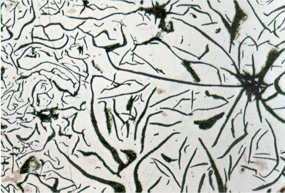
Figure 2: Microstructure of lamellar graphite cast iron material
